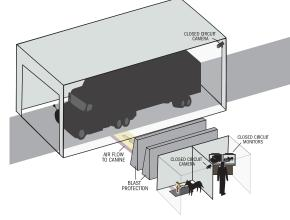
Screening rooms can be configured to allow vehicles to be screened as they pass through without being required to come to a full stop.
